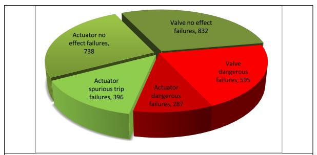
Figure 1: Typical SFF calculation for valve + actuator according to IEC 61508 first edition. The SFF is the percentage of the chart that is coloured green, which is 69%.
