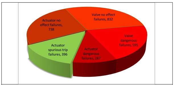
Figure 2: Typical SFF calculation for valve + actuator according to IEC 61508 second edition. This time, the SFF is only 31%.
